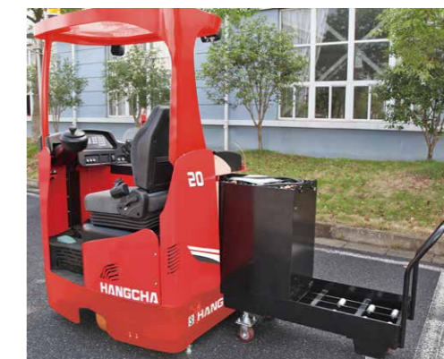
Standard configuration: Battery side roll-out + trolley(optional)
